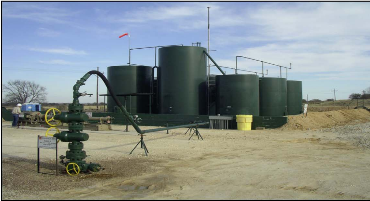
Figure 13 - Typical wellhead in Warm Climate. (GTI) No methanol or other injection equipment for freeze mitigation. Flow line is elevated without insulation or other protection from cold weather. Tank battery and other production equipment are not protected from cold weather. (Ref. 4)
